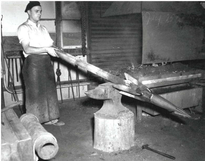
Reconditioning harpoons at the Nor' West Whaling Company, Carnarvon in 1951. (Battye Library, SLWA 008438D)
